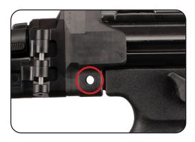
d. Install the takedown pin (two bolts are present on the MP5K) with the spring in front. Push the takedown pin through the receiver until the spring comes out on the opposite side and locks the stock.
