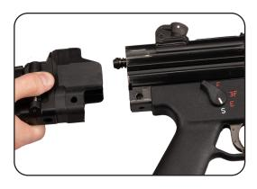
c. Use the other hand to insert the stock into the receiver. The hole in the receiver and the stock must be concentrically superimposed.
